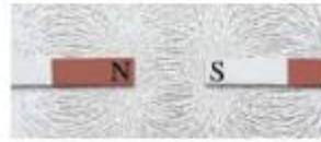
FIGURE 22.21 Iron filings sprinkled around the ends of a magnet suggest that the influence of the magnet extends into the space around it.
