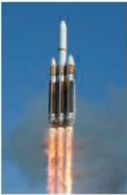
The total momentum of the rocket + gases system is conserved, so the rocket accelerates forward as the gases are expelled backward.
