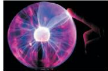
A plasma ball consists of a small metal ball charged to a potential of about 2000 V inside a hollow glass sphere. The electric field of the high-voltage ball is sufficient to cause a gas breakdown at this pressure, creating "lightning bolts" between the ball and the glass sphere.
